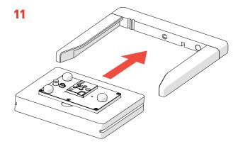
· Insert the *Pad Head* with it's protective foam case into the *Black Bay Zone*.
