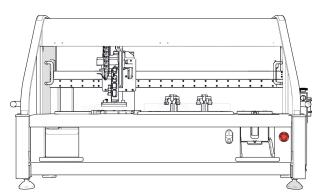
· Once the carriage arm has moved into position, turn power off ROTOR+ by pressing the *Red Stop Button*.
