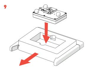
· Place the *Pad Head* into the *Foam Case*, remove from the *Black Bay Zone* and store away safely.
