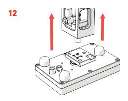
• Connect the *Pad Head* to the *Carriage Arm* by lifting it up until it snaps into place. The pneumatic connector should be on the left hand side when facing the ROTOR+.
