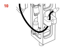
Remove the *Pad Head Gripper Contact Cable* from the holder on the carriage arm and replace it with *The Stinger Data Cable*.
