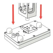
· Pull down gently on the *Pad Head* with both hands until it comes free from the *Magnetic Carriage Arm*. Remember to grip the pad head firmly.
