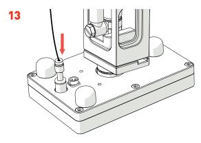
· Connect the *Pneumatic Line* to the *Pad Head* by gently inserting it into the *Pneumatic Socket*.
