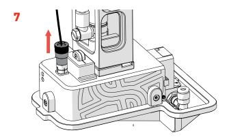
· While still holding *The Stinger*, without twisting, gently pull the *Data Cable* with your free hand by the plug, until it disconnects.
