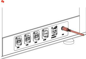
· Insert the ColonyCam power supply into the power socket on the side of the machine.
