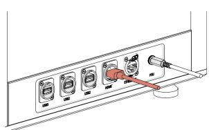
· Connect the ColonyCam to the screen using the supplied HDMI cable.
