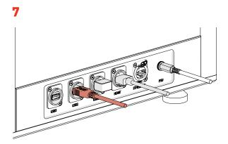
• [OPTIONAL] Attach a barcode scanner to the second USB 2.0 Socket if using.
