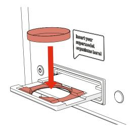
\*The provided Petri Dish Adaptor needs to be used to image 90 mm Petri Dishes.
