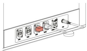
· Connect the keyboard and mouse dongle to one of the USB 2.0 sockets on the side of ColonyCam.
