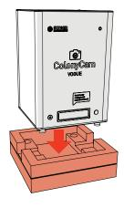
· Carefully place ColonyCam back in the lower foam and tray.
