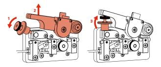
• Carefully lift the *Tension Lever* and rest it on the *Spring Catch* as shown.
