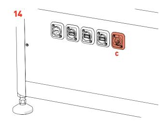
• For internal network access, connect an *Ethernet Cable* to the *RJ45 Socket (C)*.
