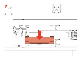
• If you have a Maldi compatible PIXL, install the removeable target bay in the Bay 2 position.
