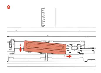
• Install the *Source Bay* by sliding the right side under the *Cleaver Tabs*, then lowering the left side onto the magnetic base.
