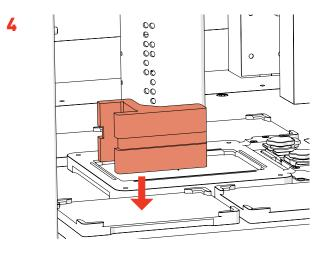
• Position the floating head in the middle of the machine and remove the transit bracket.
