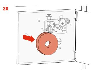
· Remove the Reel Backing Plates.
