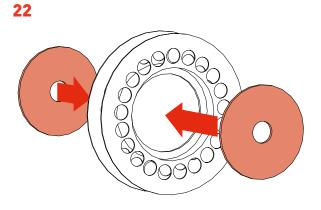
• Fit the *Reel Backing Plates* into new the *PickupLine™ Reel.*
