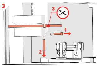
• Use *3mm Hex Key* to undo *Side Screw* (1), then remove *Securing Rod* (2). Cut the cable tie securing the floating head transit bracket with a pair of scissors (3).
