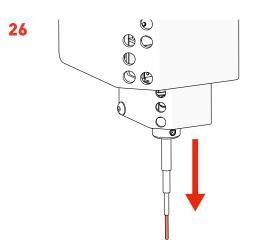
Feed the *PickupLine™* until it protrudes 10mm from the *Kinematic Nozzle*.
