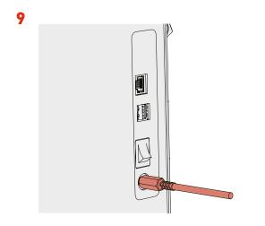
• Plug in the power supply into the wall and the power socket on the back of SQWERTY.
