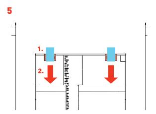
Remove the blue tape from the Door transit brackets (1) Pull both Door transit brackets with a downward motion to remove (2).
