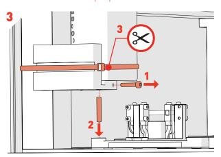
• Use 3mm Hex Key to undo Side Screw (1), then remove Securing Rod (2). Cut the cable tie securing the floating head transit bracket with a pair of scissors (3).
