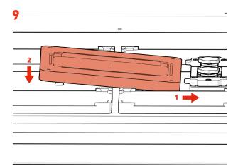
· Install the Source Bay by sliding the right side under the Cleaver Tabs (1), then lowering the left side onto the magnetic base (2).
