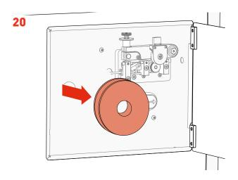
· Remove the Reel Backing Plates.
