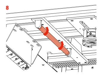
• To lock into place, turn each *UV Bulb* 90 degrees in any direction until you hear a click.
