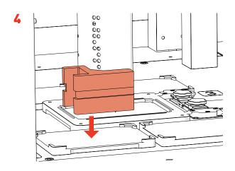
· Position the floating head in the middle of the machine and remove the transit bracket.
