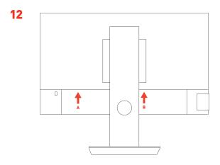
· Plug in the provided Screen cables: *Power (A) and HDMI (B)*.
