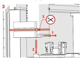
· Use 2mm Hex Key to undo Front Screw (1), then remove Securing Rod (2). Cut the cable tie securing the floating head transit bracket with a pair of scissors (3).
