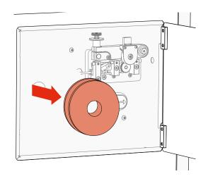
· Remove the Reel Backing Plates.
