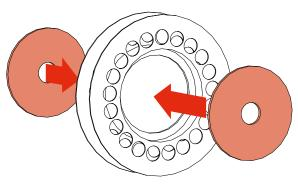
· Fit the Reel Backing Plates into new the PickupLine $^{\text{TM}}$ Reel.
