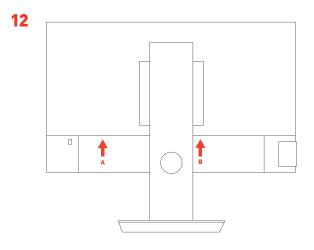
· Plug in the provided Screen cables: *Power (A) and HDMI (B).*
