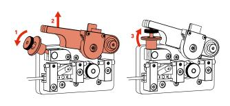
· Carefully lift the *Tension Lever* and rest it on the Spring Catch as shown.
