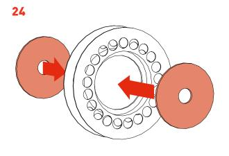
· Fit the Reel Backing Plates into new the PickupLine  $^{\text{TM}}$  Reel.
