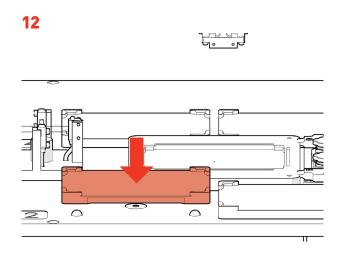
If you have a Maldi compatible PIXL, install the removeable target bay in the Bay 2 position.
