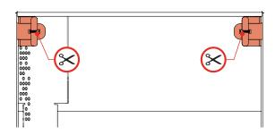
• Cut the two cable ties securing the door transit brackets with a pair of scissors.
