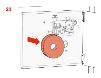
· Remove the Reel Backing Plates.
