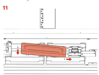
· Install the *Source Bay* by sliding the right side under the *Cleaver Tabs*, then lowering the left side onto the magnetic base.
