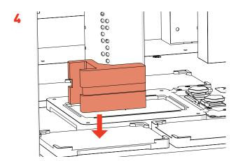
· Position the floating head in the middle of the machine and remove the transit bracket.
