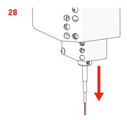
Feed the  $PickupLine^{TM}$  until it protrudes 10mm from the  $Kinematic\ Nozzle$ .
