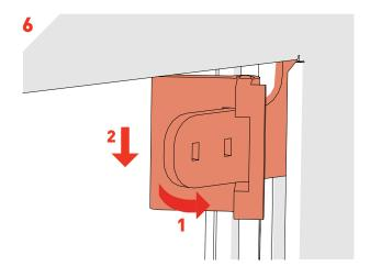
· Starting with the Right Hand Transit Bracket, open the clasp (1) and pull away from the door mechanism (2).
