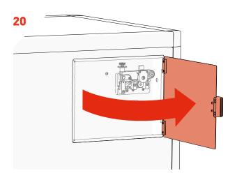
· Open the  $PickupLine^{TM}$  Compartment.
