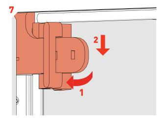
• Repeat Step 6 with the *Left Hand Transit Bracket*, open the clasp (1) and pull away from the door mechanism (2).
