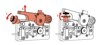
· Carefully lift the *Tension Lever* and rest it on the *Spring Catch* as shown.
