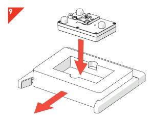
• Place the *Pad Head* into the *Foam Case*, remove from the *Black Bay Zone* and store away safely.
