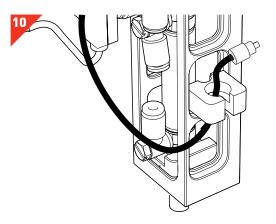
• Remove *The Stinger Data Contact Cable* from the holder on the carriage arm and replace it with the *Pad Head Gripper Contact Cable.*
