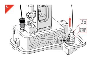
• While holding the *The Stinger* with one hand, press in the *Connection Locking Ring* with your thumb and first finger while gently pulling the *Pneumatic Connector* by the plastic shaft with your other hand.
