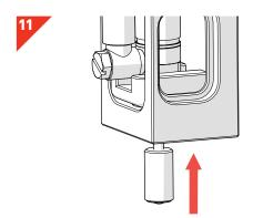
• Please ensure the *Cylinder Head* is pushed inside the *Carriage Arm Cylinder* to ensure that it is not obstructing *The Stinger* from being correctly attached.
