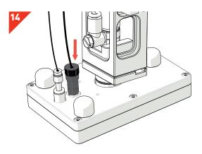
• Insert the *Pad Head Gripper Contact Cable* into the *Contact Cable Socket.*
