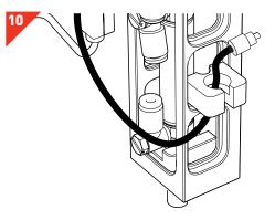
• Remove the *Pad Head Gripper Contact Cable* from the holder on the carriage arm and replace it with *The Stinger Data Cable.*
