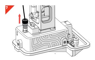
• While still holding *The Stinger*, without twisting, gently pull the *Data Cable* with your free hand by the plug, until it disconnects.
