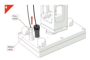
• While holding the *Pad Head* with one hand, press in the *Connection Locking Ring* with your thumb and first finger while gently pulling the *Pneumatic Connector* by the plastic shaft with your other hand.
