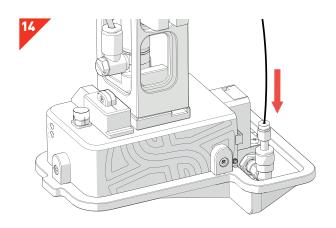
• Connect the *Pneumatic Line* to *The Stinger Head* by gently inserting it into the *Pneumatic Socket*
