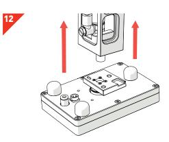
• Connect the *Pad Head* to the *Carriage Arm* by lifting it up until it snaps into place. The pneumatic connector should be on the left hand side when facing the ROTOR HDA.
