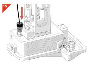
· Insert The Stinger Data Cable into Data Socket.
