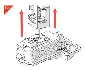
• Connect *The Stinger* to the *Carriage Arm* by lifting it up until it snaps into place. The cylinder arm should be on the right hand side when facing the ROTOR HDA (as shown).
