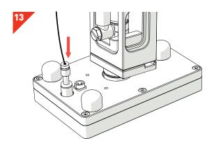
• Connect the *Pneumatic Line* to the *Pad Head* by gently inserting it into the *Pneumatic Socket*.
