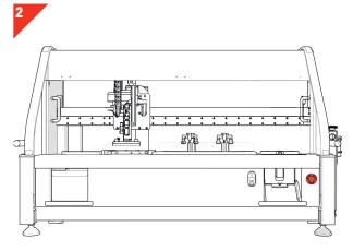
• Once the carriage arm has moved into position, turn power off ROTOR HDA by pressing *Red Stop Button*.
