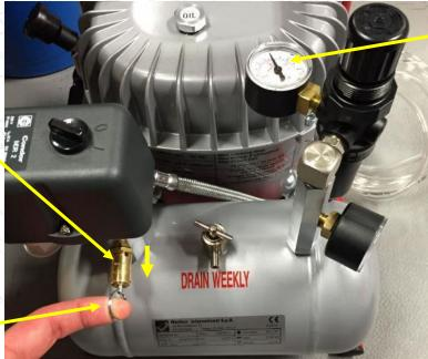
Observe pressure gauge to make sure that the needle returns to 0.
