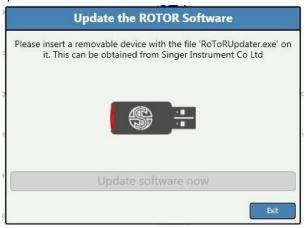
Download the software to a USB Data Key and plug the Data Key into the ROTOR MCI (computer). When the necessary files are found the 'Update Software Now' button will become active. Select and the software will be updated.
