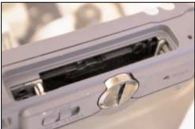
With the old card removed locate replacement.
