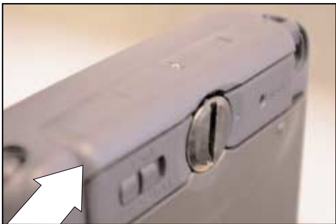
Location of the Compact Flash-Card. It may be necessary to remove the PC from the cradle
