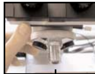
On first use ensure there is clearance between the longer objective and the dish.
