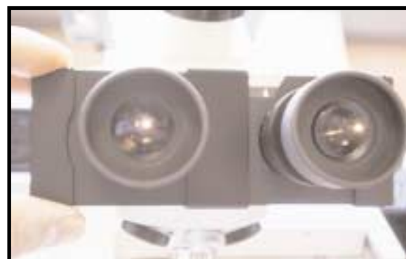
Eye width adjust is made by pulling or pushing one of the linear eyepiece tracks. Standard distance is 63 or at dot.
