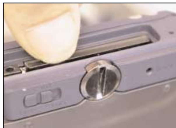
Push the Flash-Card all the way in and replace the lid.
