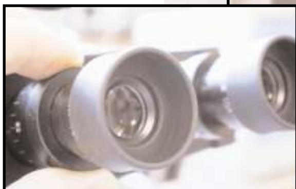
Eyepiece focusing can be made by turning the 'knurled' ring (not the rubber cup).
