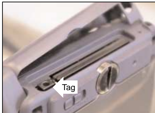
Remove the stylus and unclip the top. It will remove so be careful that it does not get misplaced. Pushing the tag down ejects the card
