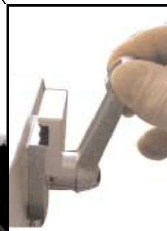
Lowering the overarm is carried out by first supporting the overarm with one hand and pulling the overarm latch-handle towards you with the other. Gently lower the arm until it stops.
