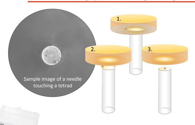
The flat surface of the **Singer Needle** without any sharp protrusions allows the tetrad to be easily picked up by a combination of capillary action and surface tension
