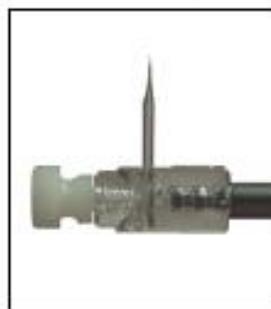
Place the tool holder in the Micromanipulator as shown.
